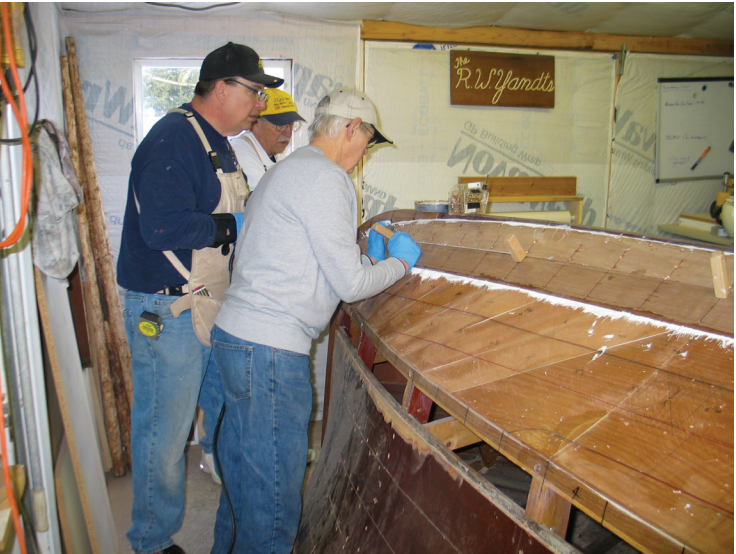
Skippy . Shown is Wes Yandt working with Glenn Dutro, on right, and Ron Yandt seating bottom planks into 3M 5200 sealant.
