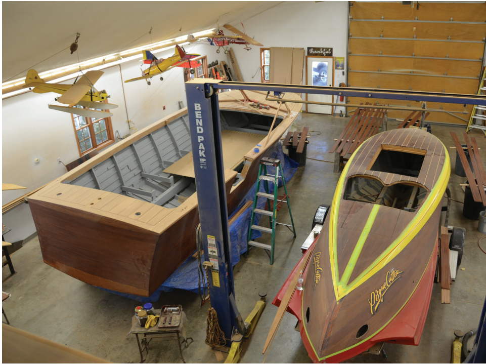
Young's newly designed 25-footer under construction is shown on the left next to a 22-foot torpedo he is reconfiguring from a four-place, engine aft speedster into a mid-engine two-seater.
