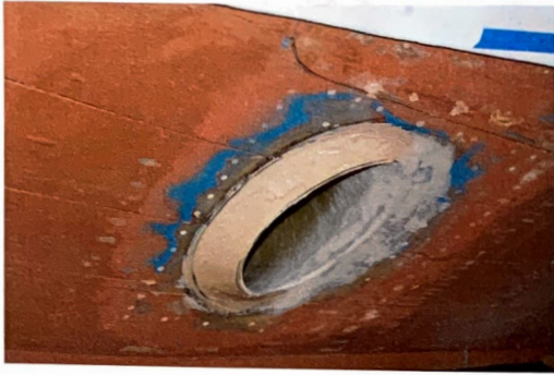
A new bow thruster, seemingly sized for a battleship, should provide excellent maneuvering.
