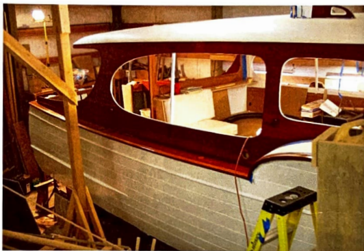
The exterior varnish was stripped, sanded, stained, sealed, and built up with new varnish. The final varnish coat is now on a good portion of the cabin exterior.
