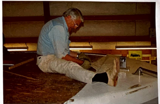
Canvas on the cabintop and deck was repaired and/or replaced.
