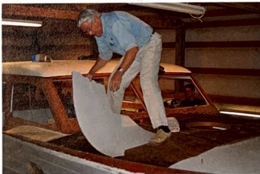
Canvas on the cabintop and deck was repaired and/or replaced.
