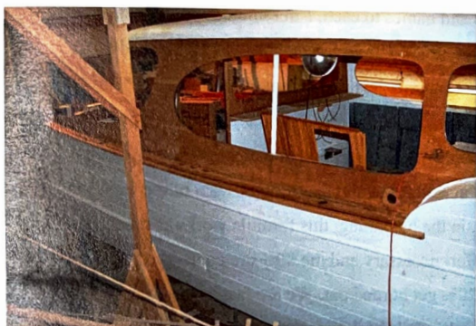
The exterior varnish was stripped, sanded, stained, sealed, and built up with new varnish. The final varnish coat is now on a good portion of the cabin exterior.
