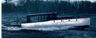
Two Pullman berths and two berths in the stern seat provide sleeping accommodations for four in the thirty-five-foot Whitney cruiser, at left. It has a galley and a gas heater. Its speed is fifteen to twenty-two miles an hour.
