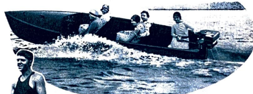
"Faybow Middy," an all-mahogany sixteen-foot outboard craft, can go thirty miles an hour and turn in almost its own length.
