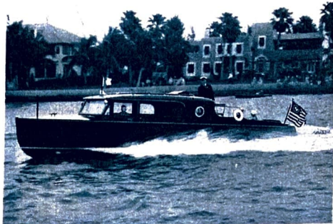
The thirty-two-foot Robinson "Seagull," one of the fastest of sedan cruisers. It makes thirty-two miles an hour. The cabin contains comfortable berths, upholstered seats, built-in lockers, and a smart little galley.
