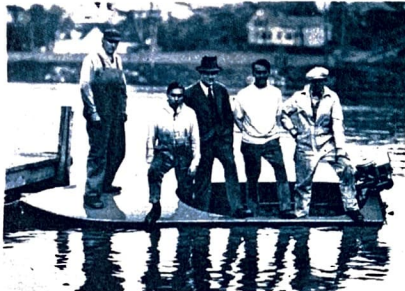
They can't sink it! A five-foot air tank in the bow of the "Baby Steelcraft," a twelve-foot outboard boat of eighteen-gage metal, is said to hold up the weight of passengers and engine in case of accident. There is not a bolt, rivet, or other fastening in the all-metal hull. It goes thirty miles an hour.
