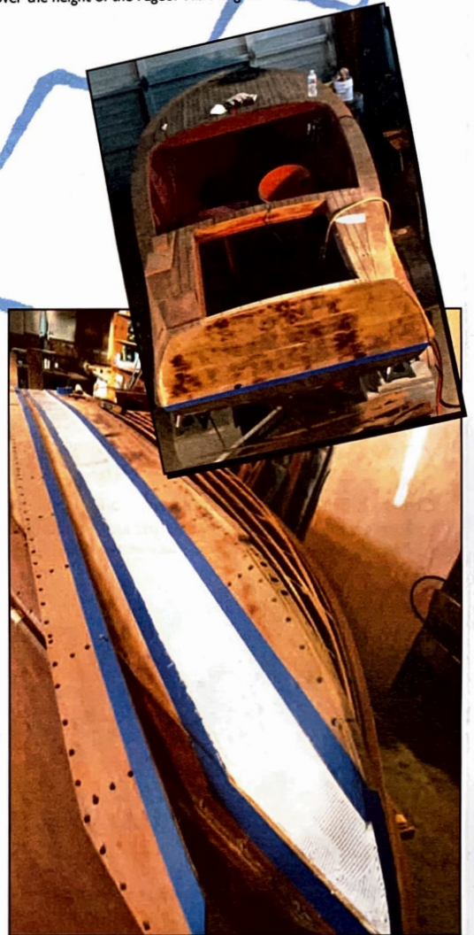
Brothers, Dick and Greg Goodell start the process of installing a 5200 bottom
