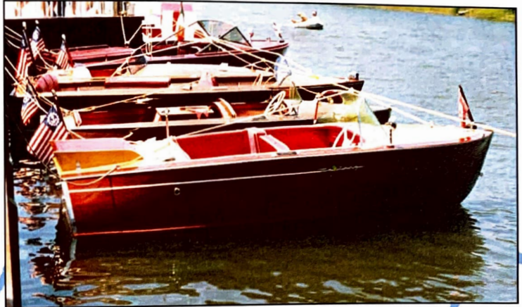
Image of a 1957 Century Colt VIP from the Century Boat Club Website. Notice the raised engine hatch on the aft deck to cover the height of the Fageol V.I.P. Engine
